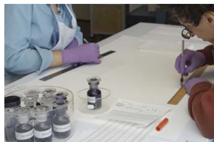
Figures 18-20. Sample preparation. Ink ingredients, above; sample inks, middle; applying inks to sample papers, bottom.
