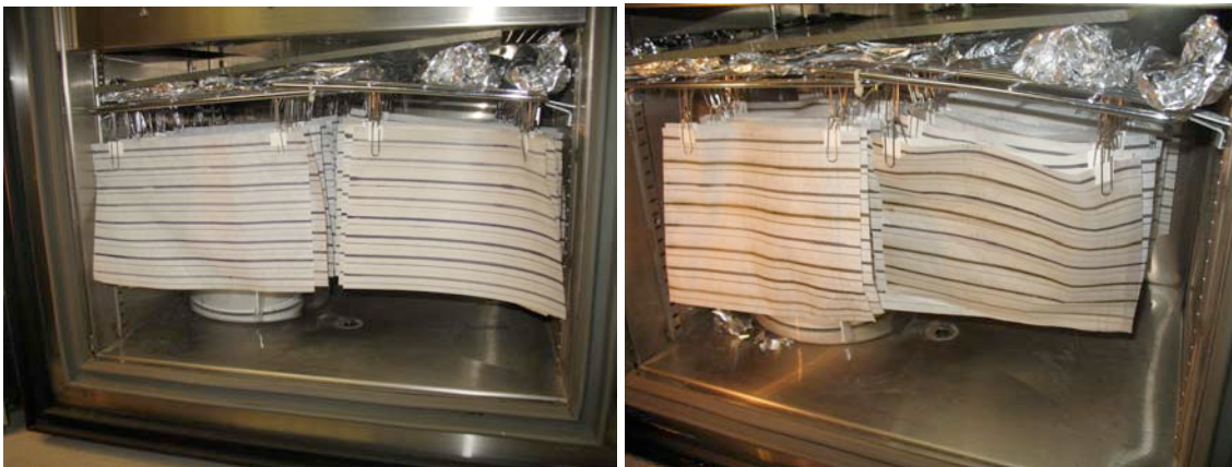
Figures 21-23. Aging samples in lab oven. Samples before (left) and after aging (right.)
