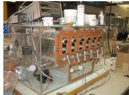
Figures 35-36. Tensiometers in climate controlled cases used for mechanical testing of paper samples.
