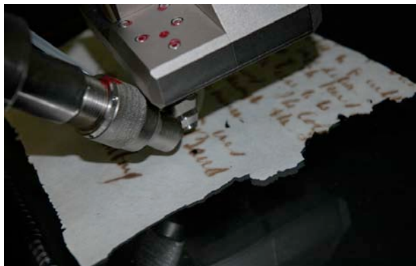
Figures 14-15. Bruker ARTAX 800 micro-XRF analyzing Baird books at MCI.
