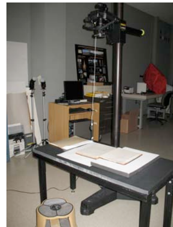
Figure 46. Digitization set-up on a copy stand with a digital camera, ring flash, and interleaving paper.
